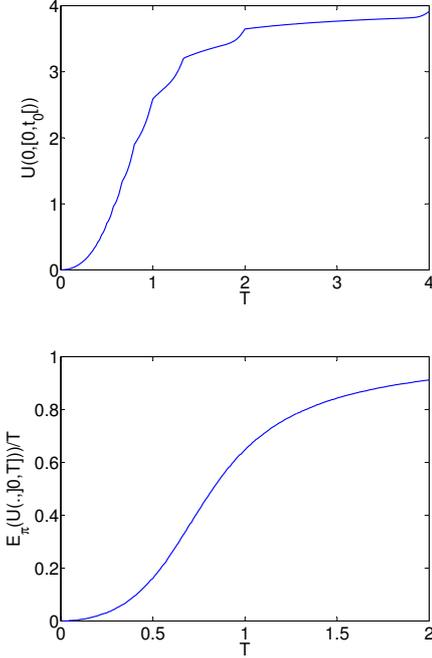
Figure 5: Mean down time in the finite horizon case (upper figure) and asymptotic unavailability (lower figure) as a function of  $T$ , Example 3
