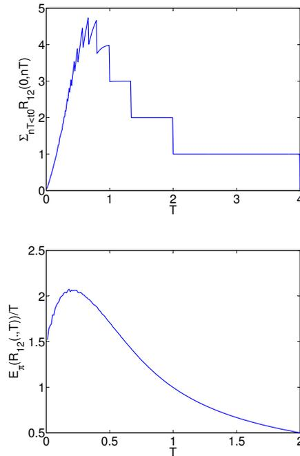
Figure 4: Mean rate (asymptotic case, lower figure) and mean number (finite time case, upper figure) of simultaneous replacements as a function of  $T$ , Example 3
